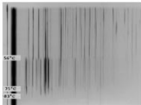
Fig. 3 Powder X-ray diffraction pattern of terpin hydrate vs. temperature
